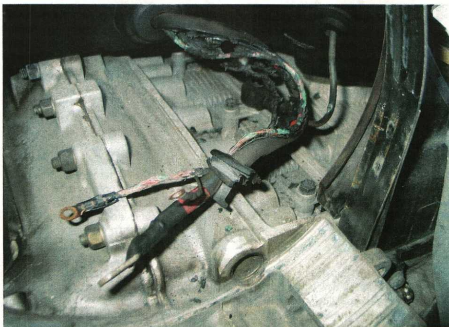
Above: This 993 engine wiring harness did not get replaced in time; the integrity of its wiring insulation has failed, allowing bare conductors to make contact.
