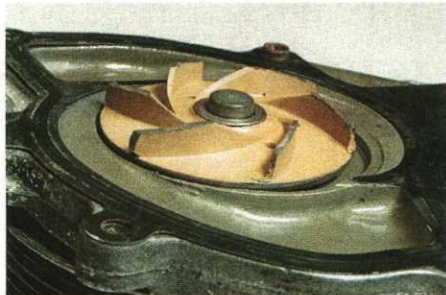
Clockwise from top left: Coolant leak from rear of Cayenne V8 and Tiptronic's torque converter area is sure sign of failed coolant pipes. Metallic fragments found in M96/996 oil filter. Worn M96 water pump. Manometer tests for crankcase vacuum; high reading indicates failing M96 air/oil separator.
