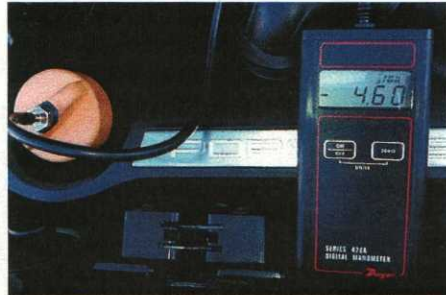
Clockwise from top left: Coolant leak from rear of Cayenne V8 and Tiptronic's torque converter area is sure sign of failed coolant pipes. Metallic fragments found in M96/996 oil filter. Worn M96 water pump. Manometer tests for crankcase vacuum; high reading indicates failing M96 air/oil separator.
