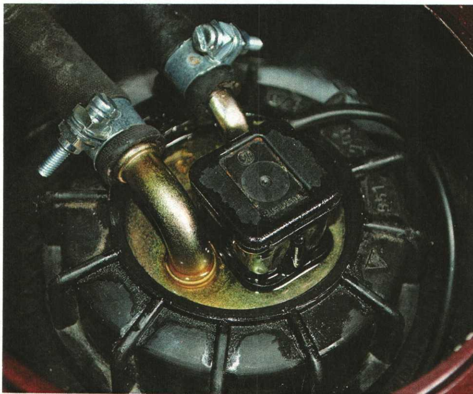
Gasoline can pool around the fuel-level sending unit (left), making the interior smell, but vent hoses in the rear storage area on the passenger side "hump" are the most likely source of gasoline fumes inside a 924/944/968. Remove the carpeting and the cover panel to access the hoses.
