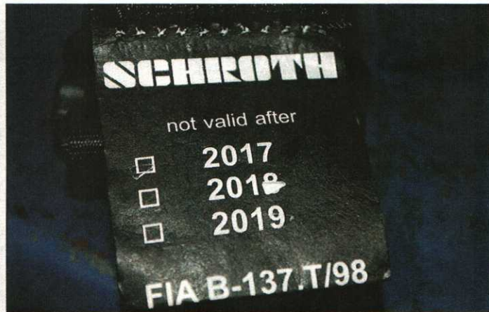
Above left: Technician checking for play in the ball joint of right rear diagonal link. Above right: Schroth seatbelt harness code and expire date.
